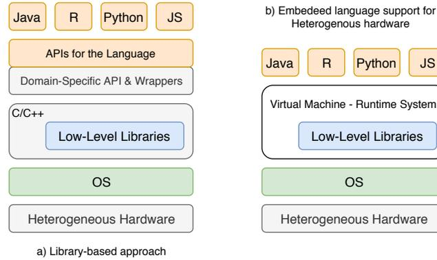
Figure 4: Software stack for running applications implemented in managed programming languages for two different approaches. The approach a) shows how currently high-level programming languages can make use of heterogeneous hardware via native APIs. The approach b) shows a different strategy in which the underlying runtime and virtual machine, that abstract the program from the hardware details, can automatically make use of the heterogeneous hardware.
