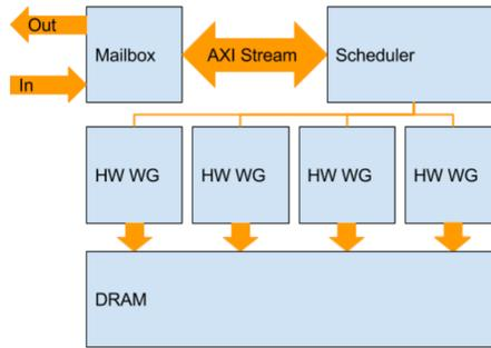
Figure 5: Overview of the virtualization block and its interfaces.
