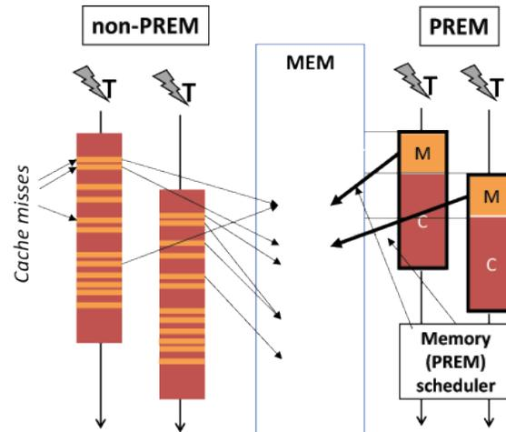
Figure 7: **PR**edictable **E**xecution **M**odel in a parallel environment.
