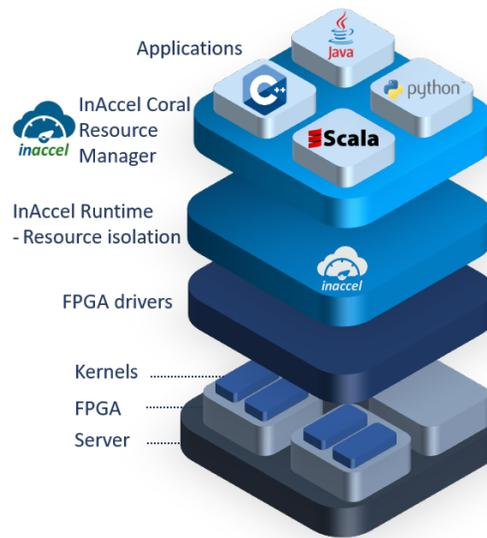
Figure 8: High-level overview of the Coral FPGA resource manager
