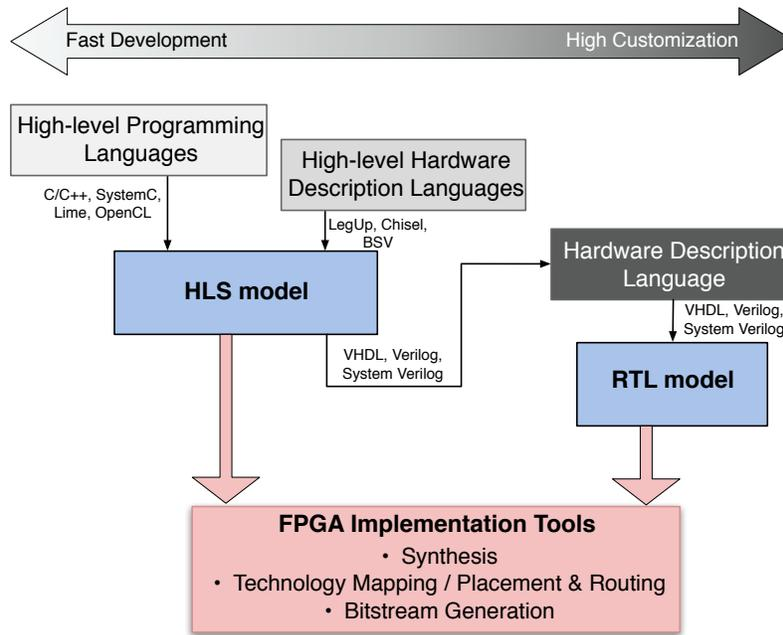
Figure 2: Programming Abstractions in Reconfigurable Computing.
